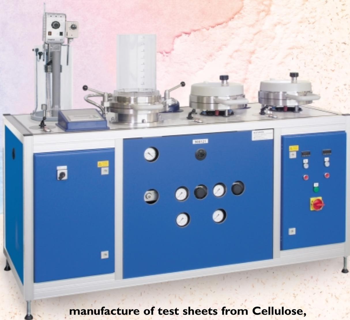
manufacture of test sheets from Cellulose,
