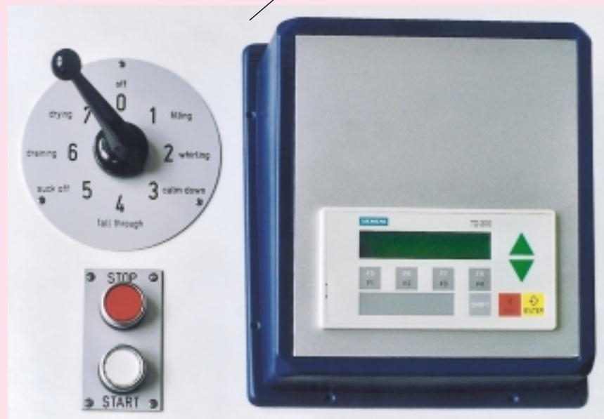
BBS-Operation Controls and Panel with Display of the Sheet Forming Column
